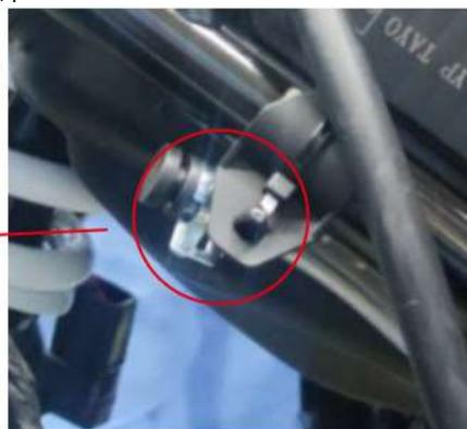
**Vela de ignição**
